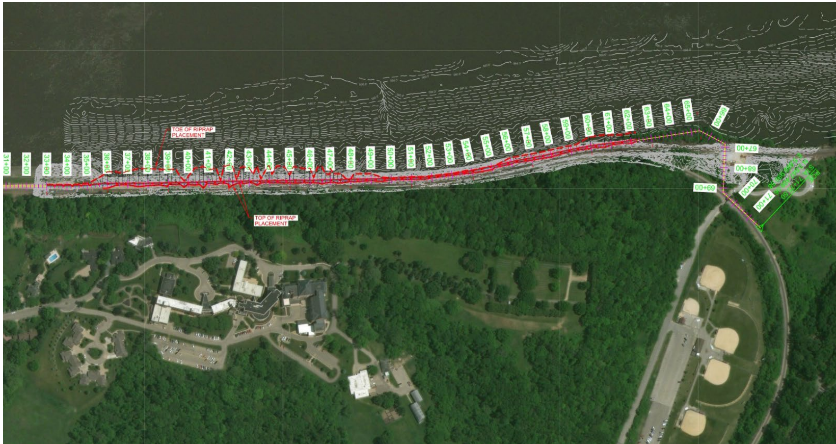
Figure C-1. Locations of Proposed Riprap Revetment
